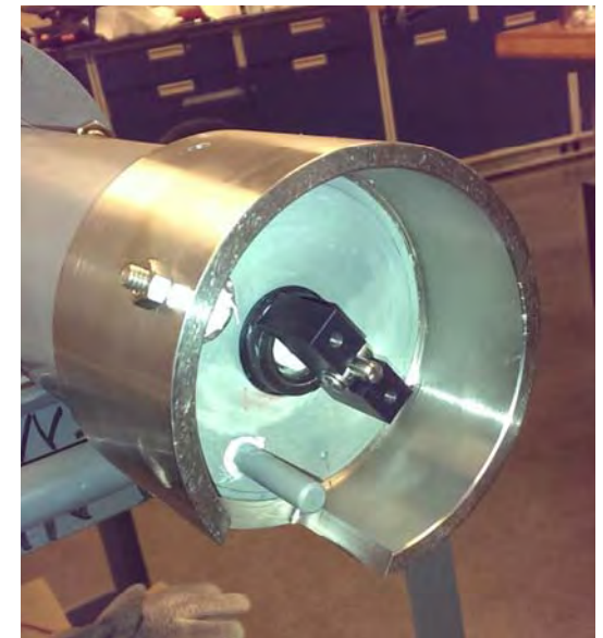
Wetted electrode/ring with rotating cleaning block for slurry service
