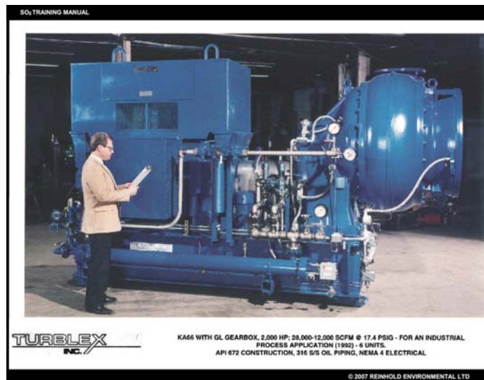
Compressor - 2000 HP Used with permission from Turbalex
