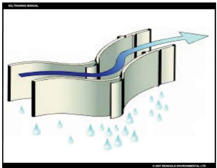
Mist Eliminator Horizontal Flow Diagram Used with permission from Munters Corp.
