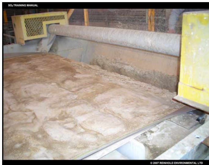
Horizontal Belt Filter - Cake Discharge Used with permission
