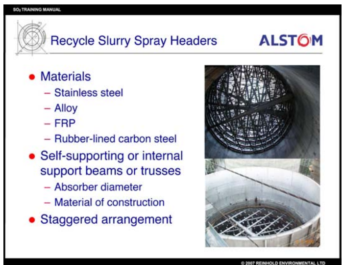
Recycle Slurry Spray Headers Used with permission from Alstom
