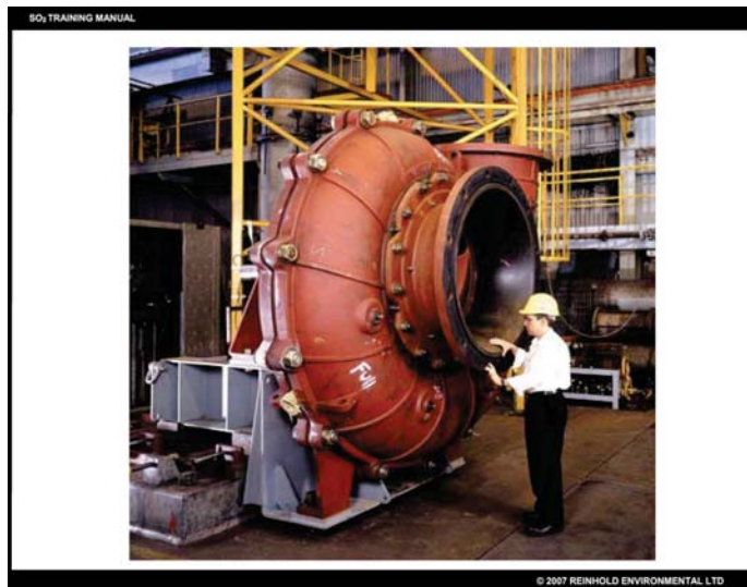
Slurry Pump Casing (FRP with Rubber Lining)
