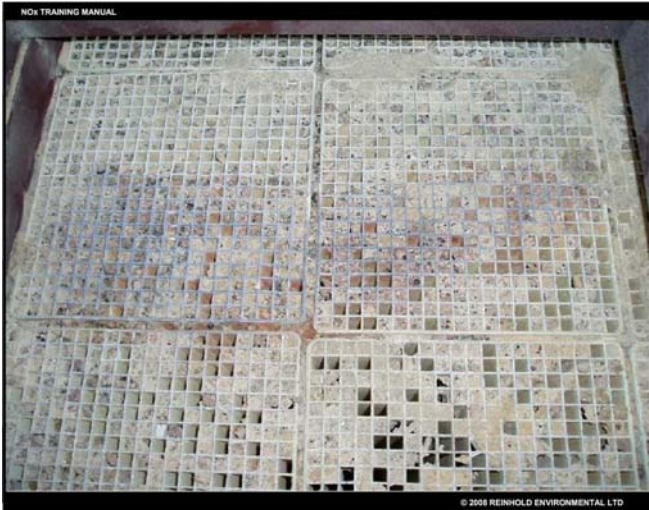
Dirty Charred Honeycomb Catalyst - 2 (Used with permission)
