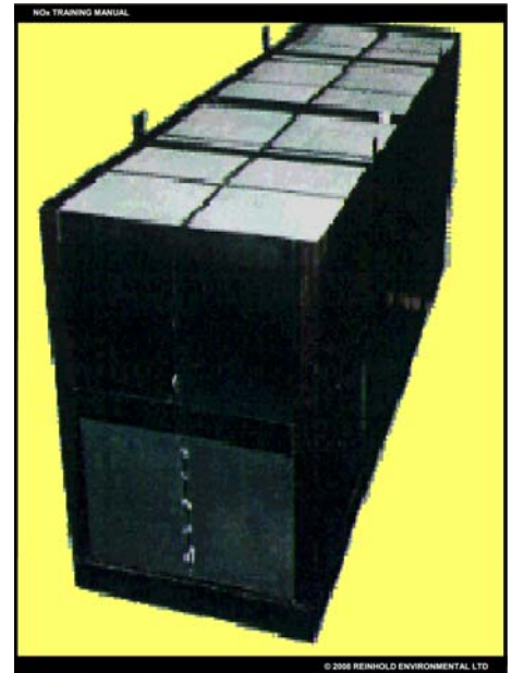
Blocks Loaded into Final Catalyst Module-Ready for Installation (Used with permission)
