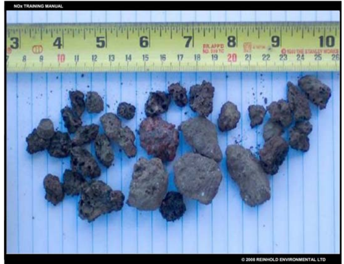
LPA (Courtesy of Evonik Energy Services)
