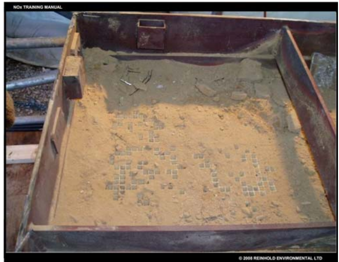
Dirty Honeycomb Catalyst - 1 (Used with permission)
