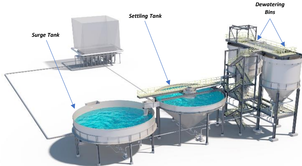
Traditional Recirculation System – Dewatering Bins with Surge/Settling Tanks
