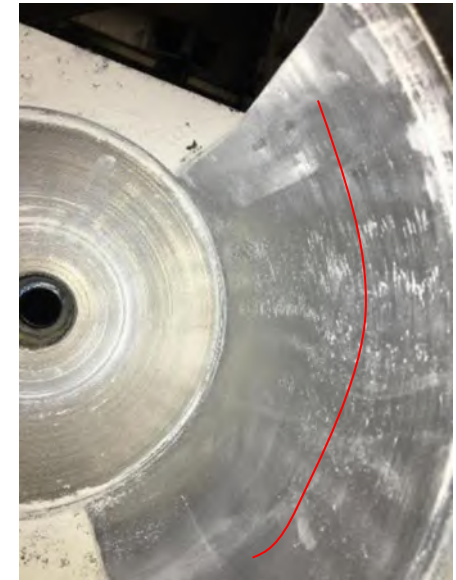
Barrel grooves can form
