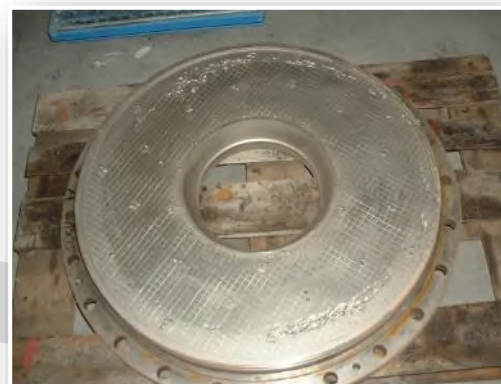
③ Welding Support Mesh/Molds
